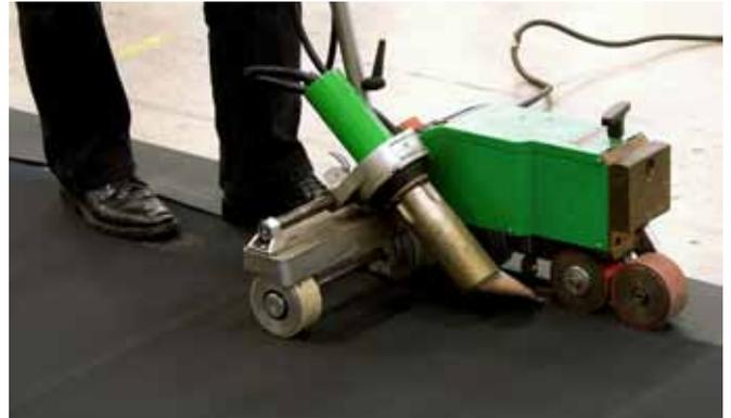
The Thermobond splice strip shall be welded with Leister Varimat.
