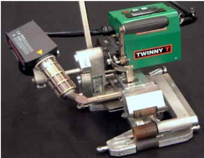
Leister Twinnny adapted with prefabrication kit are used for splicing Elastoseal T. Leister Twinnny with 50 mm rolls set up for prefabrication without test channel is SealEco article 55999021.
